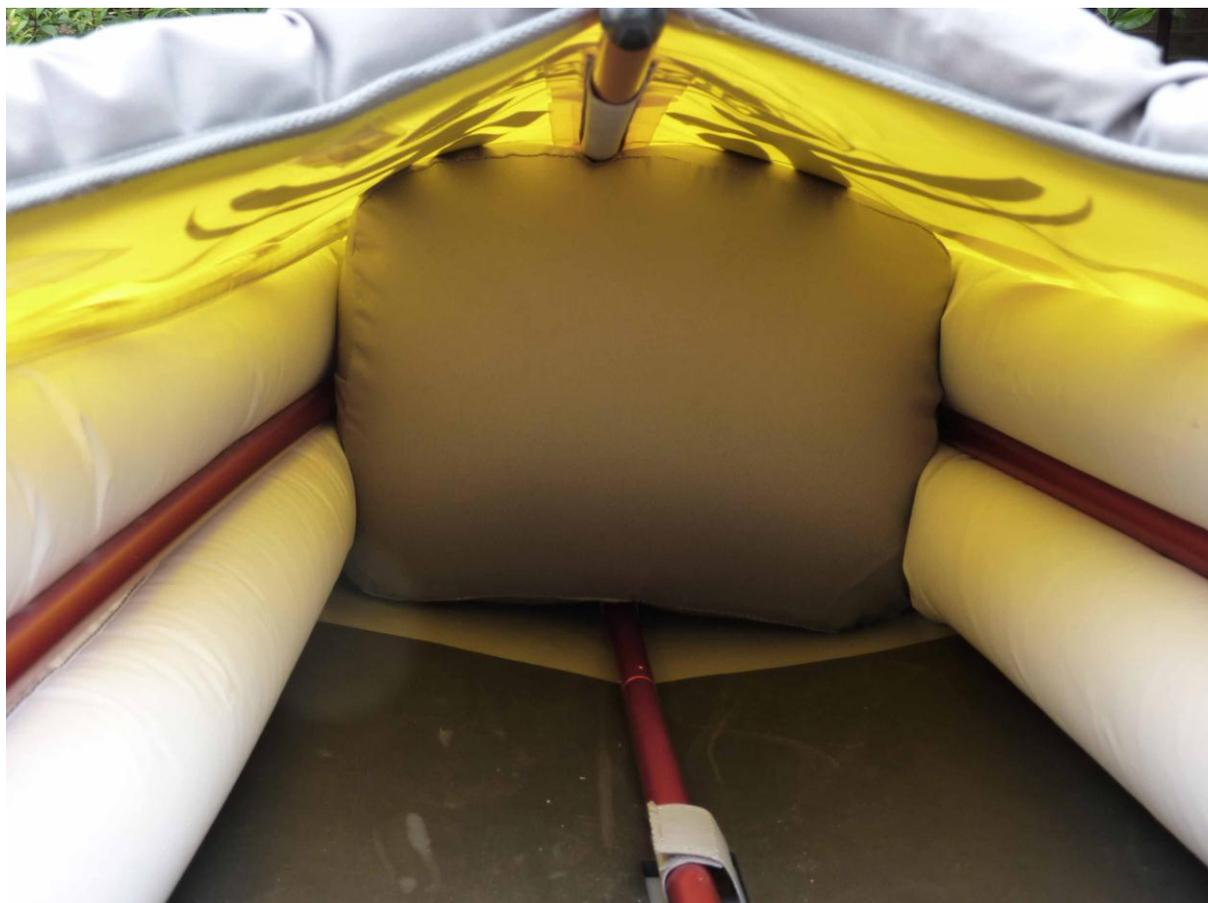
Figure 2 Showing keel tubes, front thwart, side poles between the side air tubes and front deck tube.
